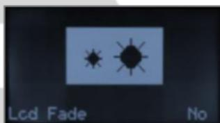
LCD Fade is used to extend 3rdH Player battery life.
