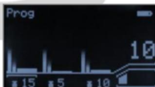
This takes you to "Ramps". A Ramp is a slow, progressive increase in sensation level. Set the amount of increase which will be added to the current sensation level. Then set the amount of time it should take.
